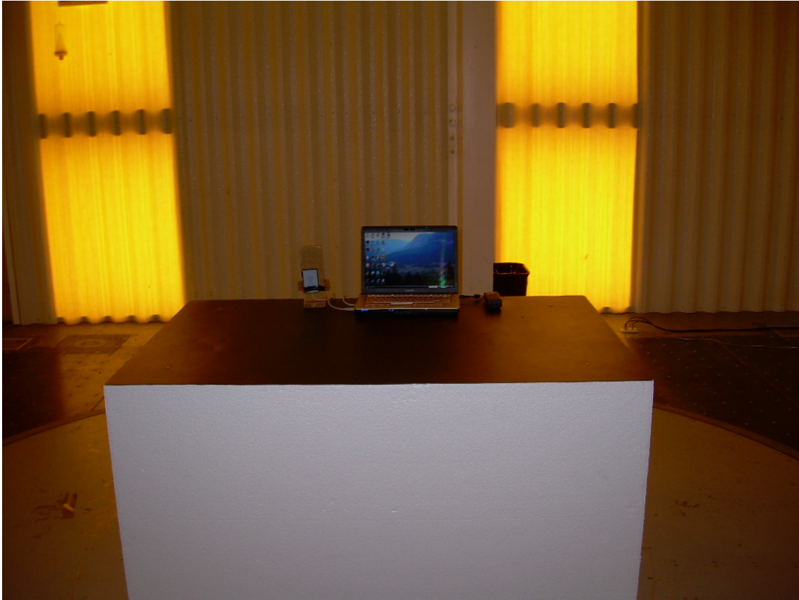
Front View Radiated Test Setup - Vertical EUT Placement
