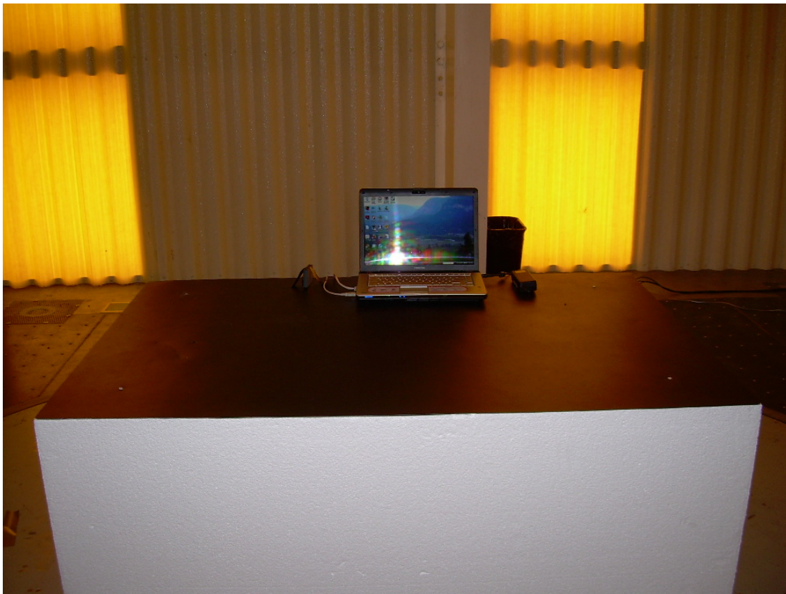
Front View Radiated Test Setup - On-Edge EUT Placement
