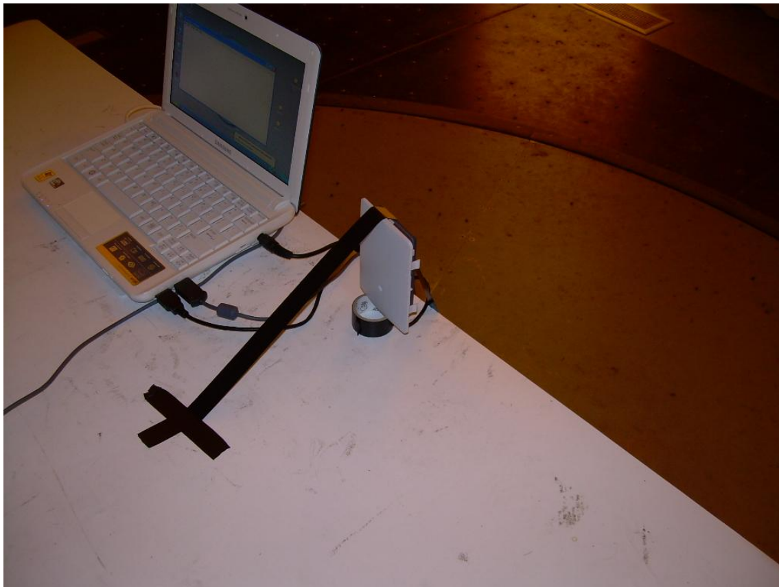
Photograph 4 – Front View Radiated Emission Setup – Vertical Placement Using Longest Cable Worst-Case Radiated Emission Configuration
