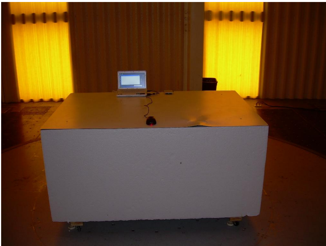
Photograph 1 – Front View Radiated Emission Setup – Horizontal Placement
