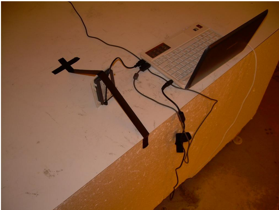
Photograph 5 – Front View Radiated Emission Setup – Vertical Placement Using Short Cable
