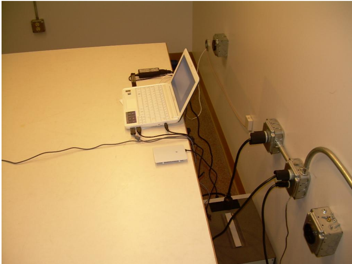
Photograph 8 – Back View Conducted Emissions at the AC Mains Setup
