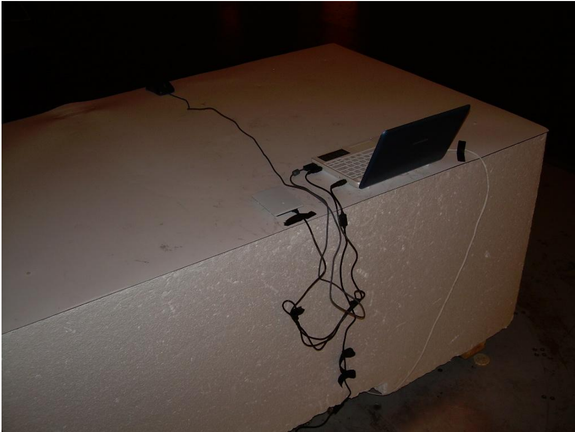
Back View Radiated Test Setup - Horizontal EUT Placement
