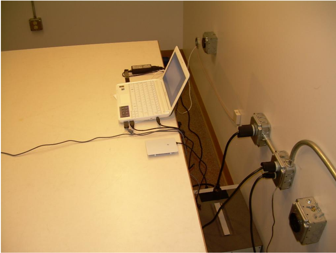
Back View Conducted Emissions at the AC Mains Setup
