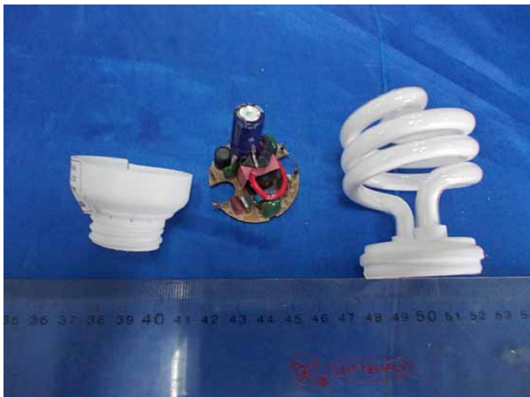
FIGURE 1 FLUORESCENT SELF-BALLASTED LAMPS (M/N: T2 HALF SPIRAL CFL - 13W) COVER REMOVED
