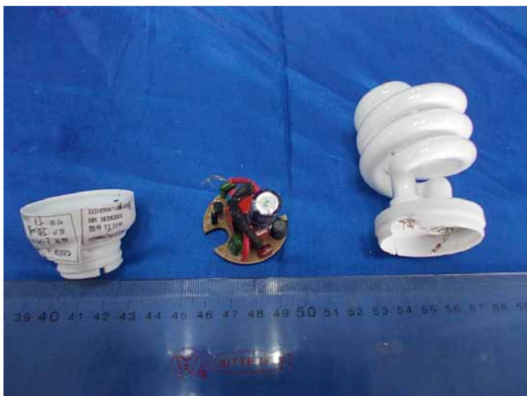
FIGURE 10 FLUORESCENT SELF-BALLASTED LAMPS (M/N: T3 HALF SPIRAL CFL - 13W) COVER REMOVED
