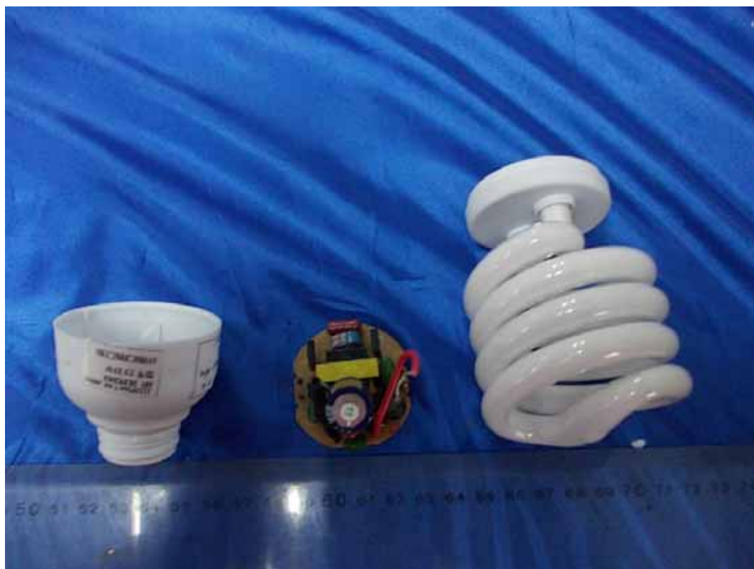
FIGURE 16 FLUORESCENT SELF-BALLASTED LAMPS (M/N: T3 HALF SPIRAL CFL - 23W) COVER REMOVED
