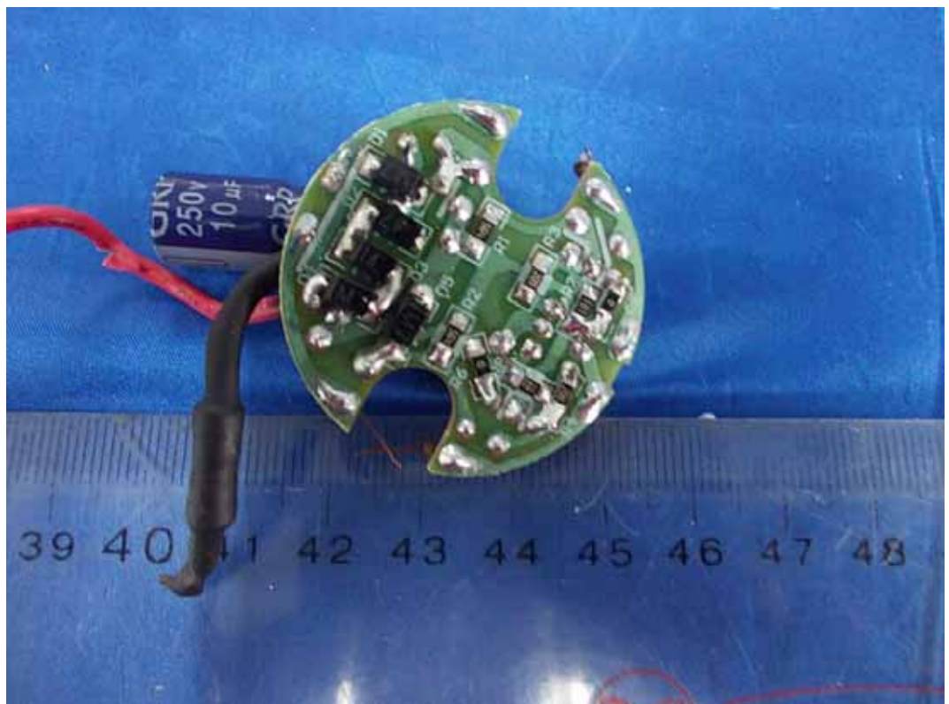
FIGURE 3 FLUORESCENT SELF-BALLASTED LAMPS (M/N: T2 HALF SPIRAL CFL - 13W) MAIN BOARD (SOLDERED SIDE)
