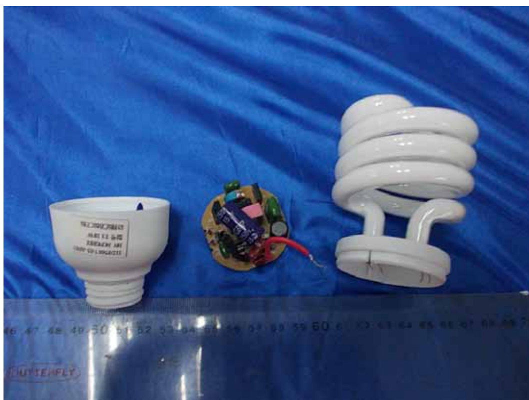
FIGURE 13 FLUORESCENT SELF-BALLASTED LAMPS (M/N: T3 HALF SPIRAL CFL - 18W) COVER REMOVED
