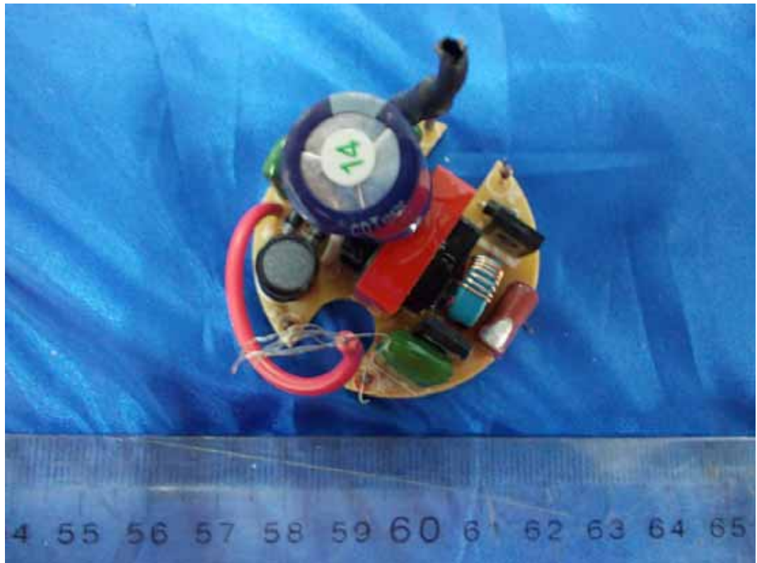
FIGURE 8 FLUORESCENT SELF-BALLASTED LAMPS (M/N: T2 HALF SPIRAL CFL - 23W) MAIN BOARD (COMPONENT SIDE)
