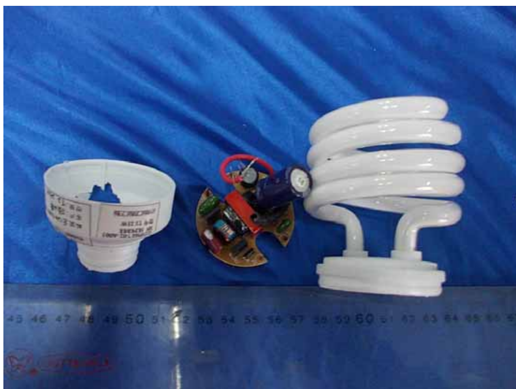
FIGURE 7 FLUORESCENT SELF-BALLASTED LAMPS (M/N: T2 HALF SPIRAL CFL - 23W) COVER REMOVED
