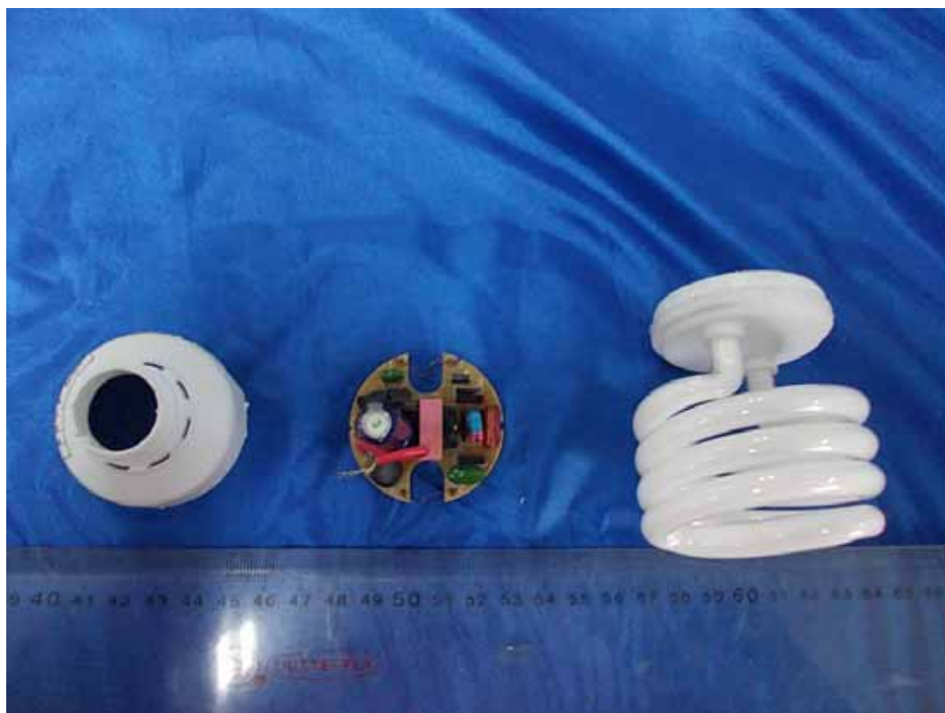
FIGURE 4 FLUORESCENT SELF-BALLASTED LAMPS (M/N: T2 HALF SPIRAL CFL - 18W) COVER REMOVED
