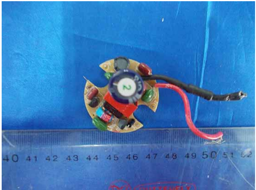
FIGURE 11 FLUORESCENT SELF-BALLASTED LAMPS (M/N: T3 HALF SPIRAL CFL - 13W) MAIN BOARD (COMPONENT SIDE)
