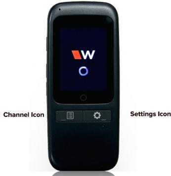
The WaveCAST Receiver can be used by audience members to listen to WaveCAST audio instead of a personal device. This can be useful for assistive listening, which has minimum in-house device requirements, or for listeners who cannot or do not want to install the WaveCAST app on their phone.
