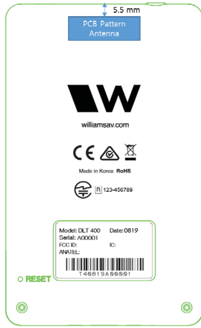
Figure F-1 Antenna Location
