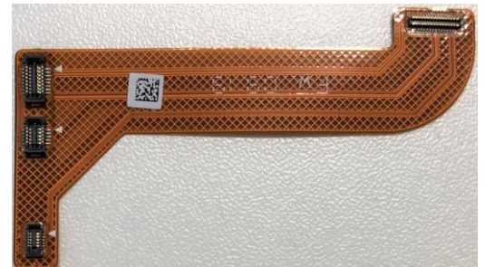
340-27174-000 ASSY, FPC, LCD JUMPER-Back, SPCC1
