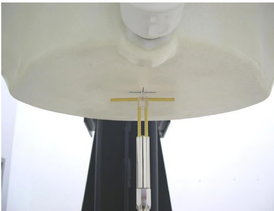
Picture 8.2 Photo of Dipole Setup
