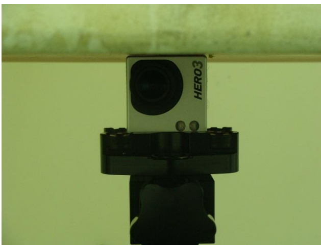
Right Side of the DUT with Phantom 0 cm Gap
