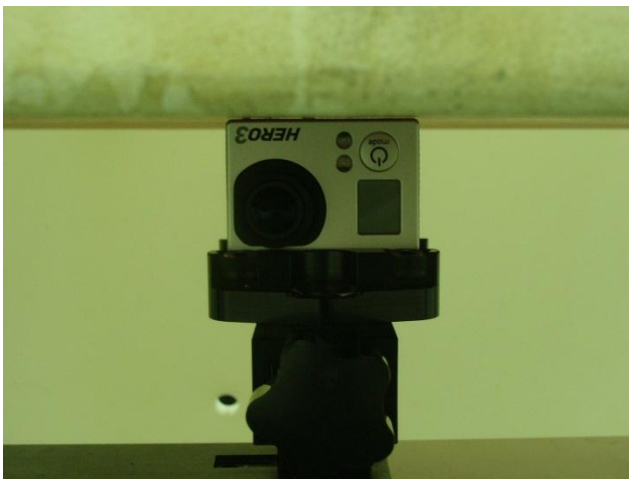
Bottom Side of the DUT with Phantom 0 cm Gap
