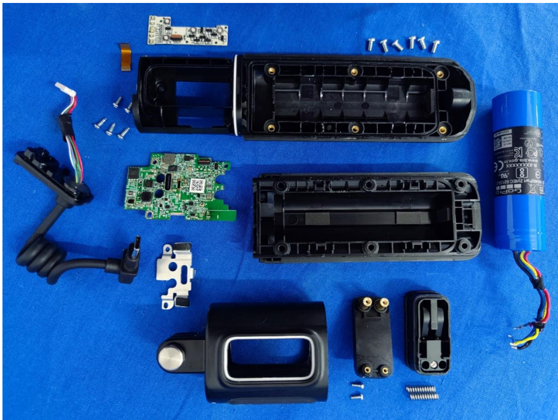
Three finger, button enclosure, battery, USB cable and all PCBA removed, ACVT1
