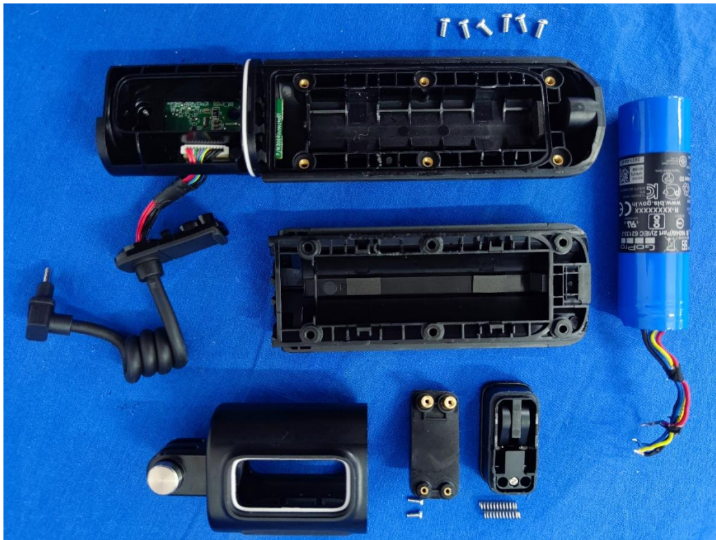
Three finger, button enclosure, Li-ion Rechargeable Battery Pack and USB cable removed, ACVT1
