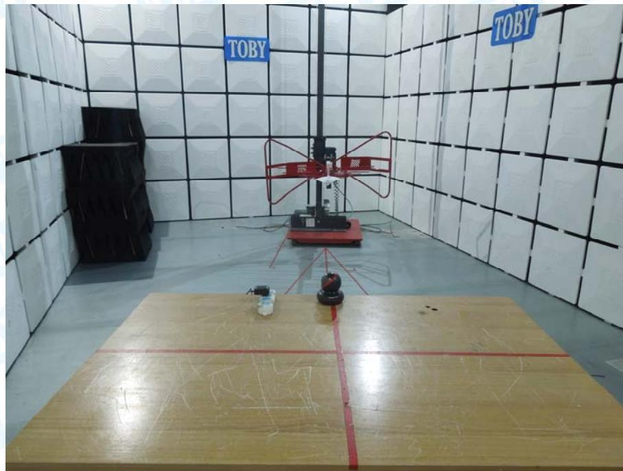
**Photo of Setup for Conducted Emission**
