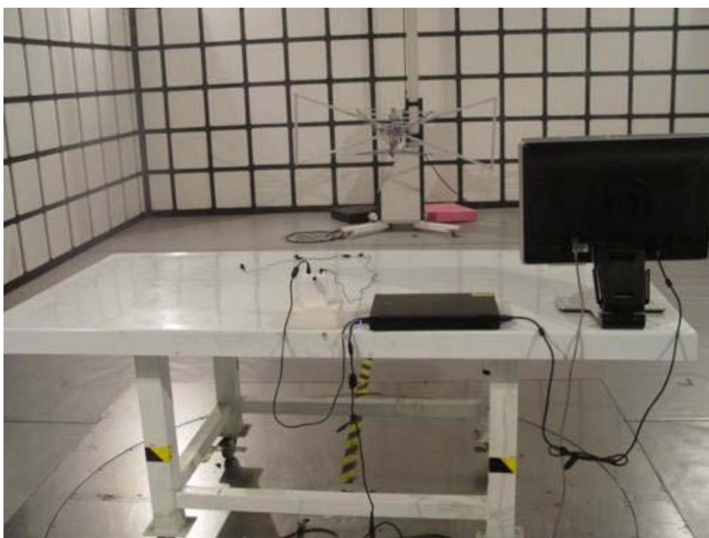
**FCC Part15B Radiated Emission above 1GHz****Setup 1- EUT+ Battery + Earphone + LCD monitor+ Notebook+ Adapter****-Front**
