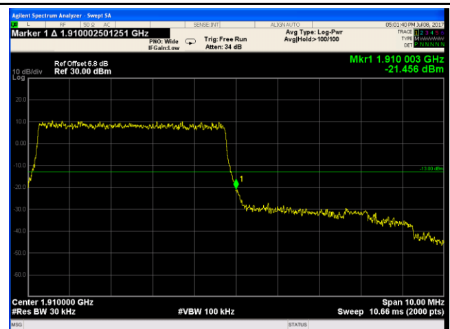
LTE band II - High Channel QPSK-5
