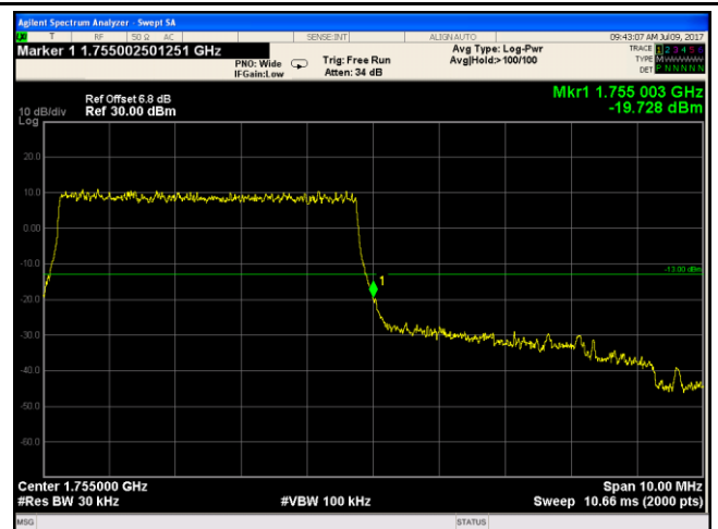
LTE band IV - High Channel QPSK-5
