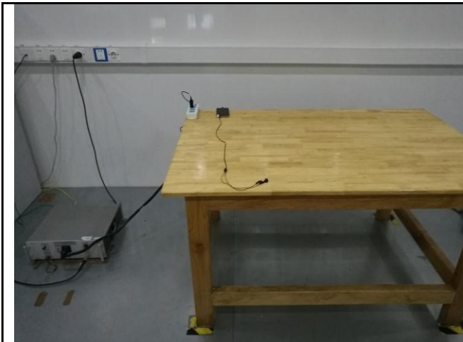
Conducted Emissions Test Setup Front View
