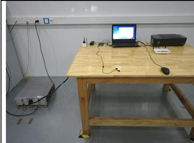
Conducted Emissions Test Setup – Front View
