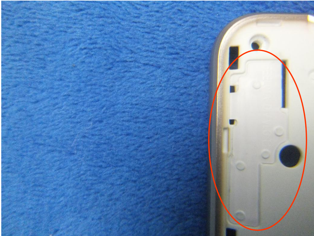
LTE - Antenna View
