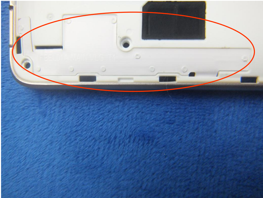
GSM/PCS/UMTS-FDD Antenna View
