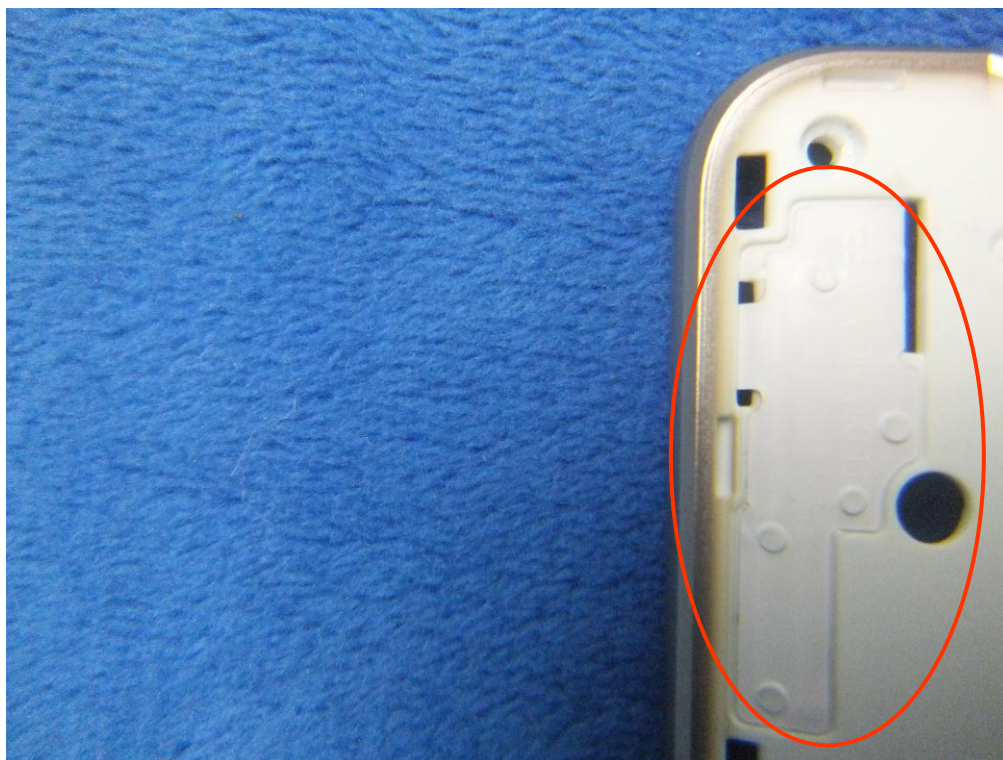
LTE - Antenna View
