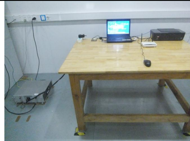
Conducted Emissions Test Setup – Front View
