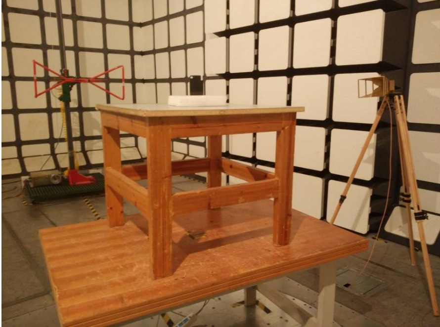
Radiated Emissions Test View (Below 1 GHz)
