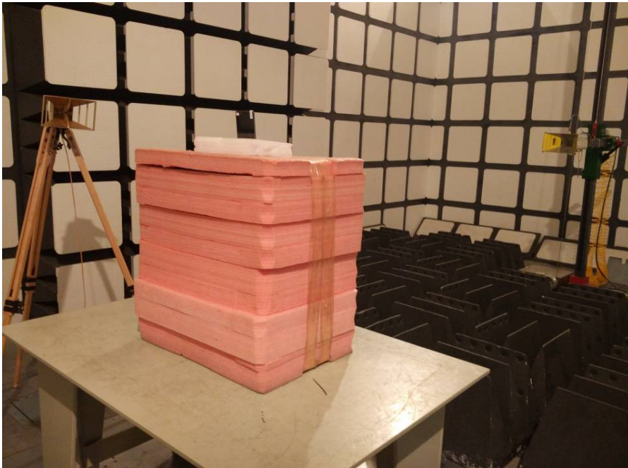
Radiated Emissions Test View (Above 1 GHz)
