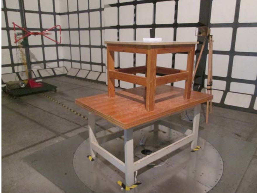
Radiated Emissions Test View (Below 1 GHz)
