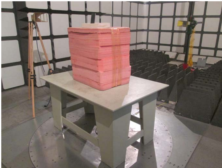
Radiated Emissions Test View (Above 1 GHz)
