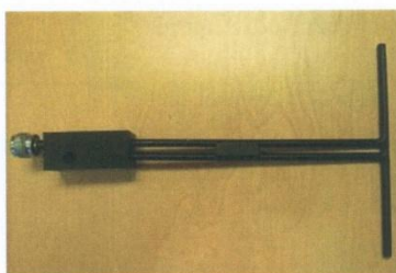
Figure 1 – MVG COMOSAR Validation Dipole
