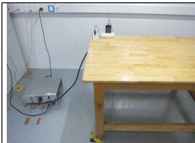
Conducted Emissions Test Setup Front View
