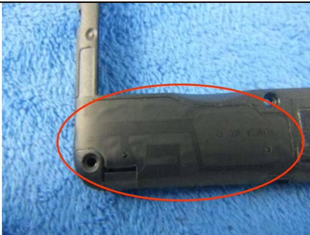
GSM/PCS/UMTS-FDD/LTE Antenna View
