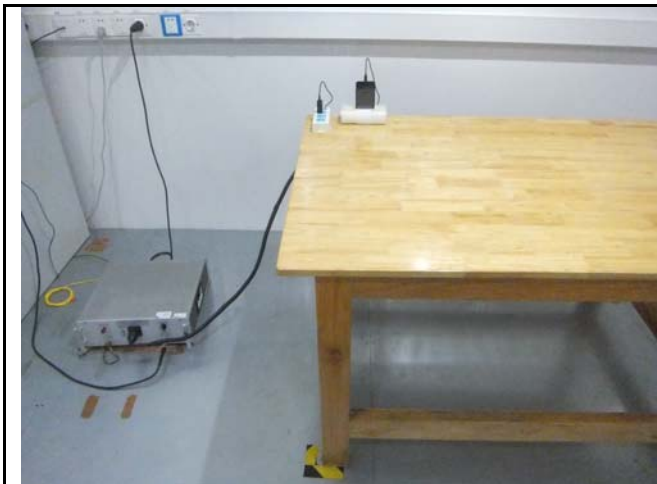
Conducted Emissions Test Setup Front View
