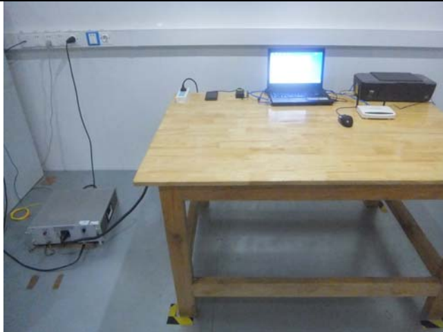
Conducted Emissions Test Setup – Front View
