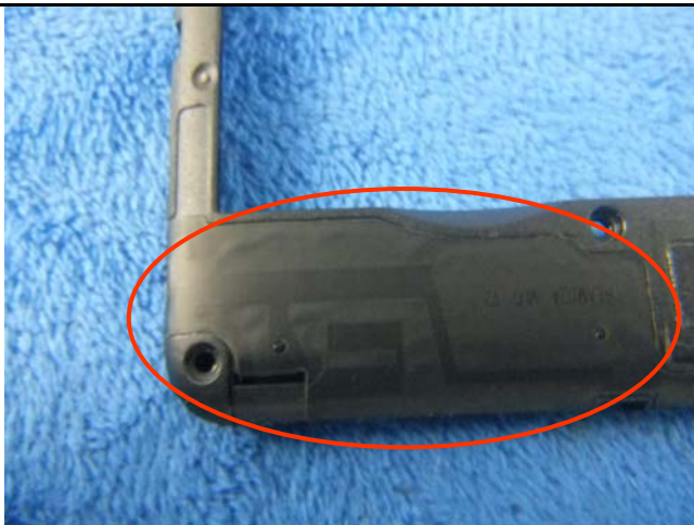
GSM/PCS/UMTS-FDD/LTE Antenna View
