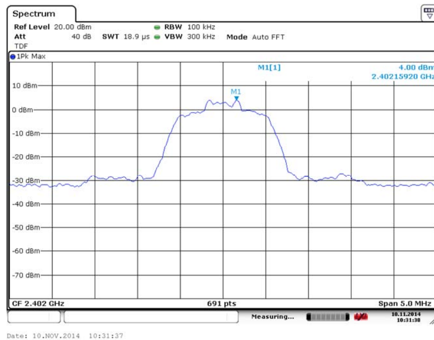
Fig. 31 Conducted Spurious Emission ( \pi/4 DQPSK, Ch0, 2.402GHz)
