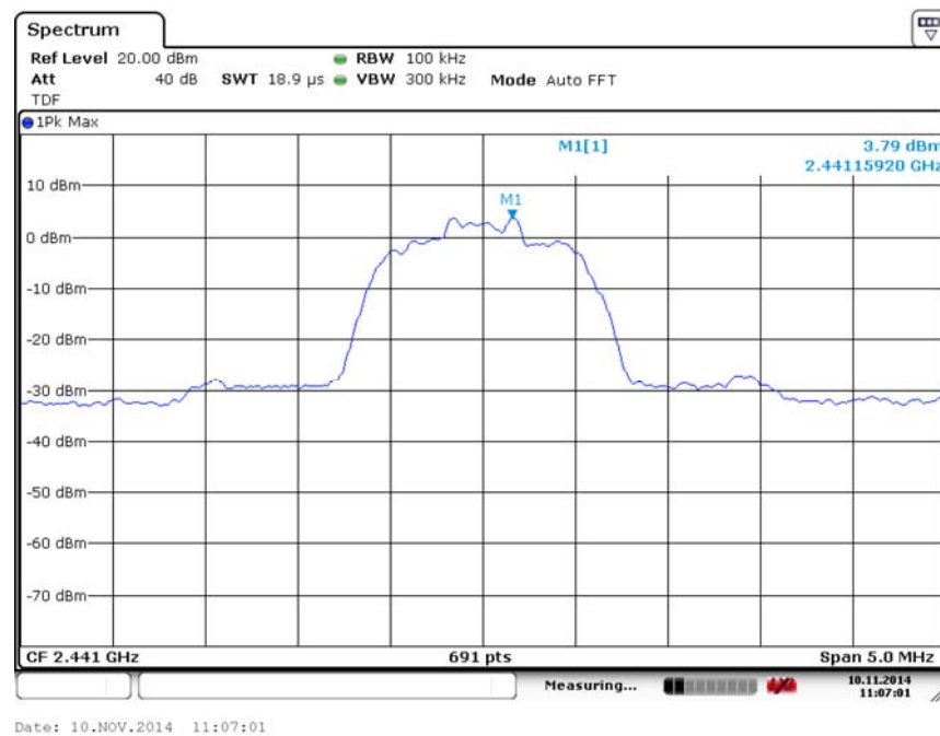
Fig. 43 Conducted Spurious Emission (8DPSK, Ch39, 2.441GHz)
