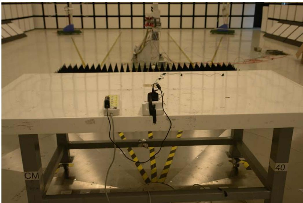
**AC Conducted Emission Test Setup**
