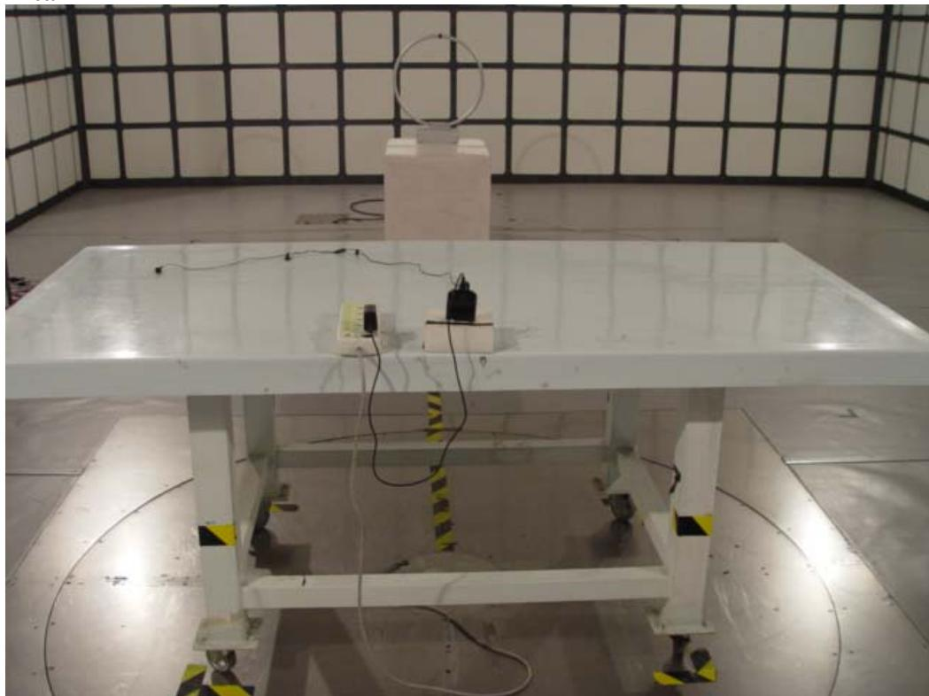
**FCC Part15C Radiated Emission below 1GHz****- Front**
