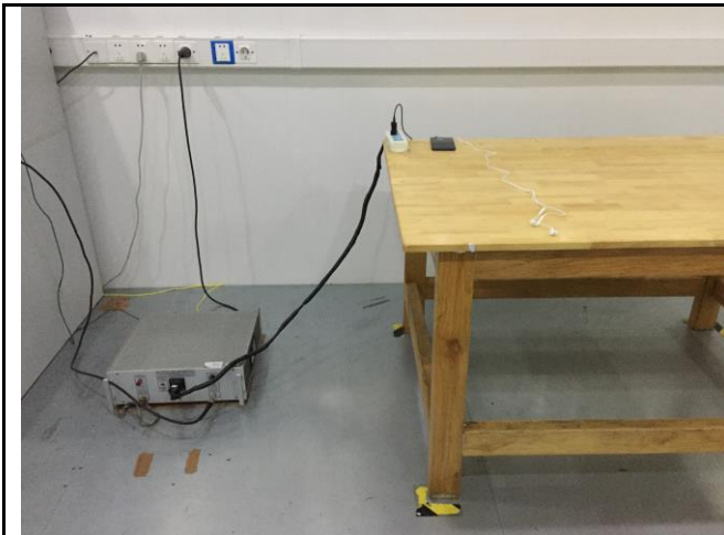
Conducted Emissions Test Setup Front View
