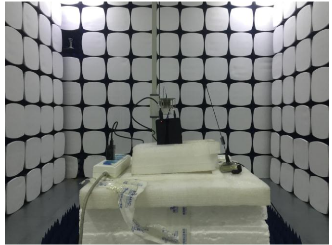
Radiated Spurious Emissions Test Setup Above 1GHz
