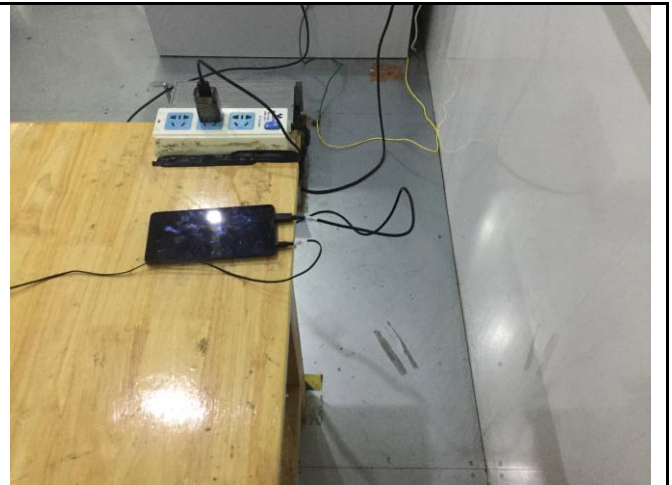
Conducted Emissions Test Setup Side View
