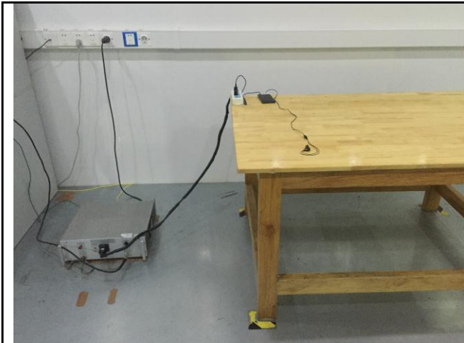
Conducted Emissions Test Setup Front View
