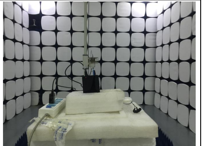
Radiated Spurious Emissions Test Setup Above 1GHz
