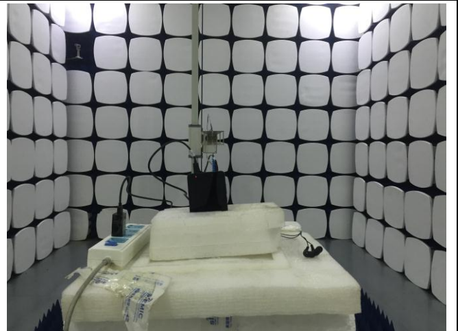
Radiated Spurious Emissions Test Setup Above 1GHz
