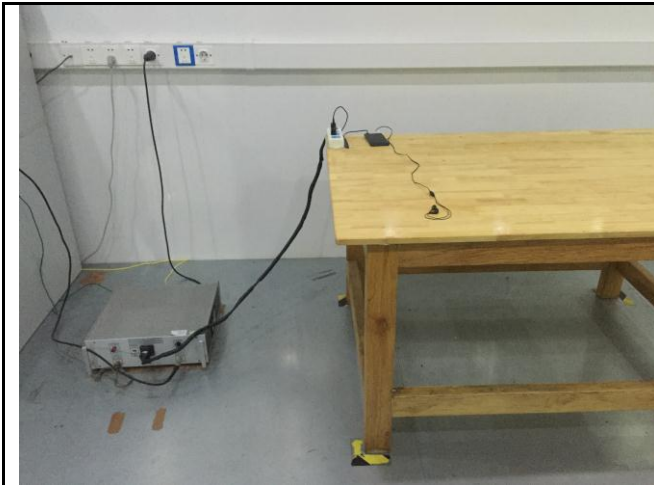
Conducted Emissions Test Setup Front View
