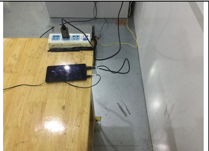
Conducted Emissions Test Setup Side View
