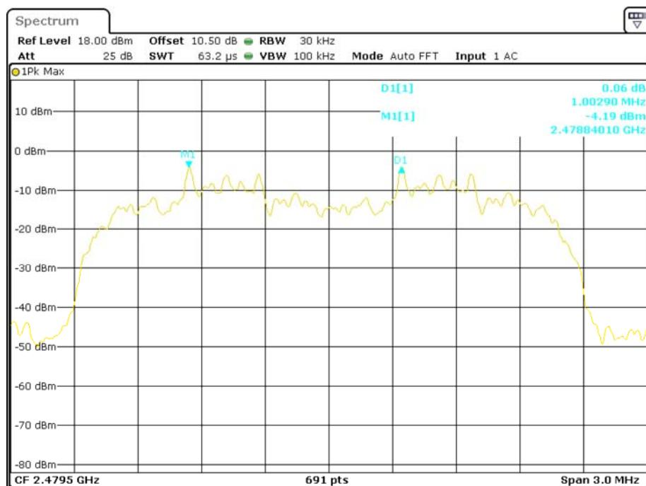
**EDR (8DPSK): Low Channel**
