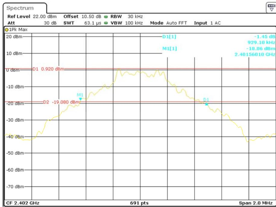
**BDR (GFSK): Middle Channel**
