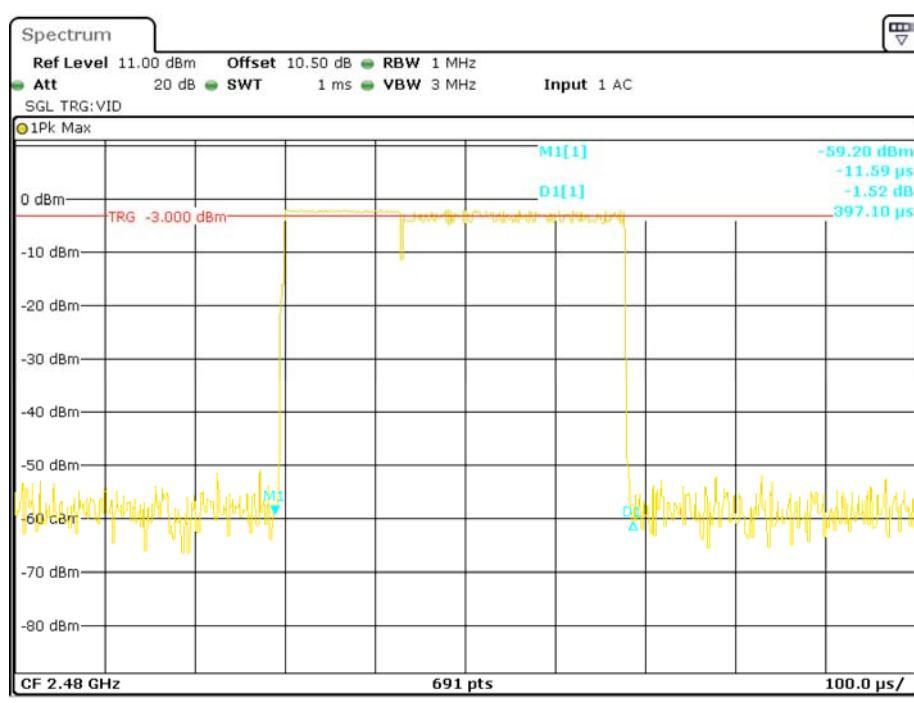
**Pulse time, Low Channel, 2DH3**
