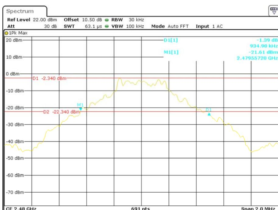
EDR ( $\pi/4$ -DQPSK): Low Channel
