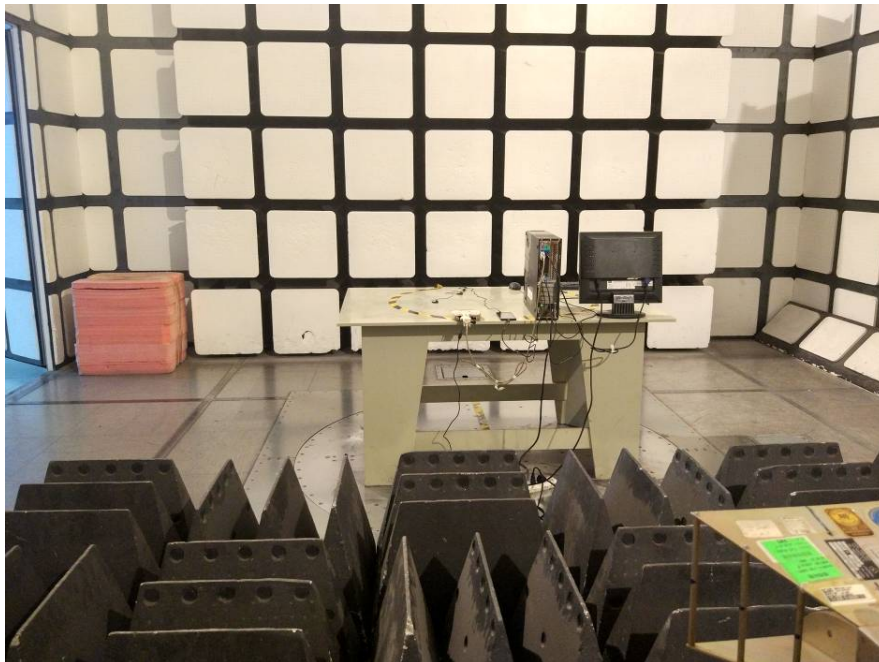
Radiated Emissions – Rear View (Above 1 GHz)
