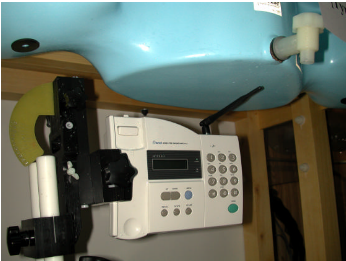
Figure 11. Test setup of EUT in normal operating position with the source of significant emissions (antenna) 2.5 cm below the phantom.
