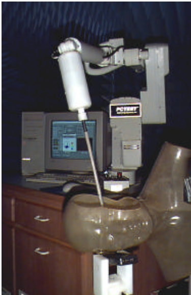
Figure 5. Photograph of the Probe and the Phantom
