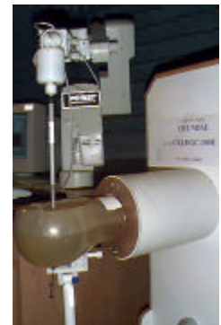
Fig. 1 SAR Test Setup
