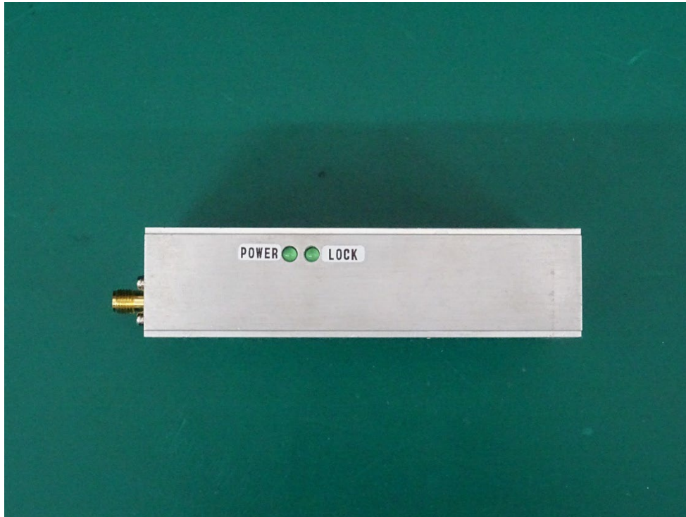
Oscillator Module (1 st Local/CGH-450) LED side view
