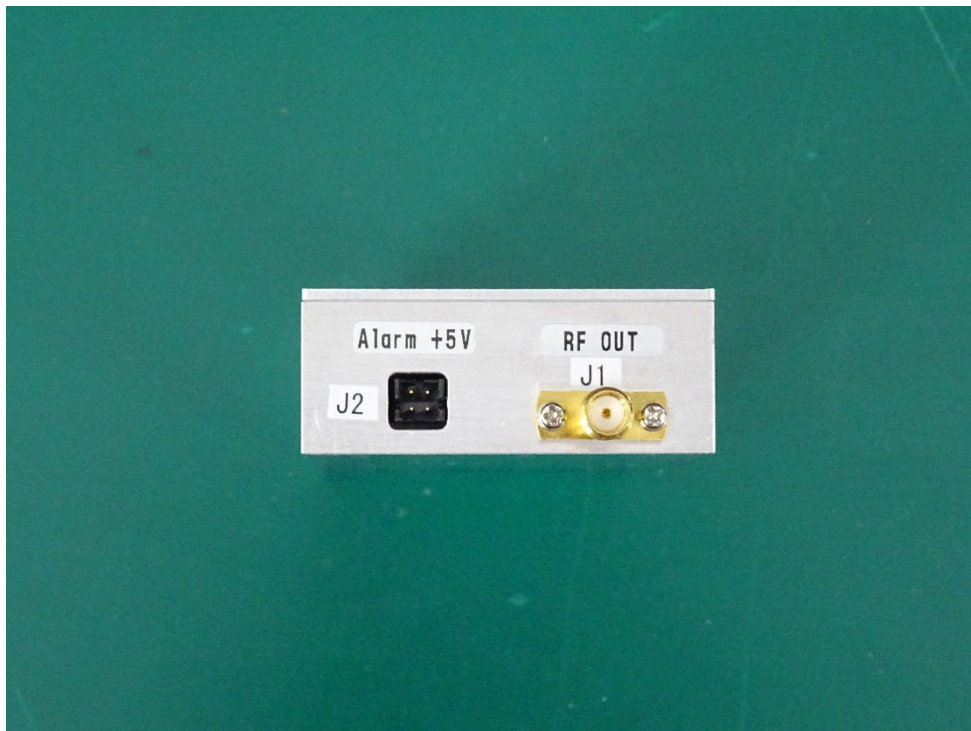
Oscillator Module (2 nd Local/CGH-382A) Connector side view
