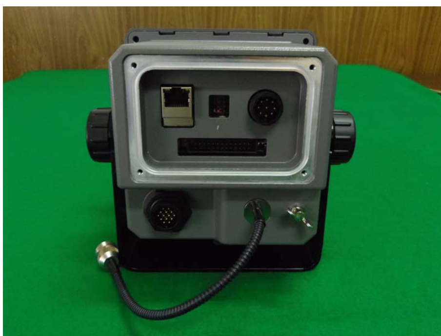
AIS Controller, Rear Panel Removed
