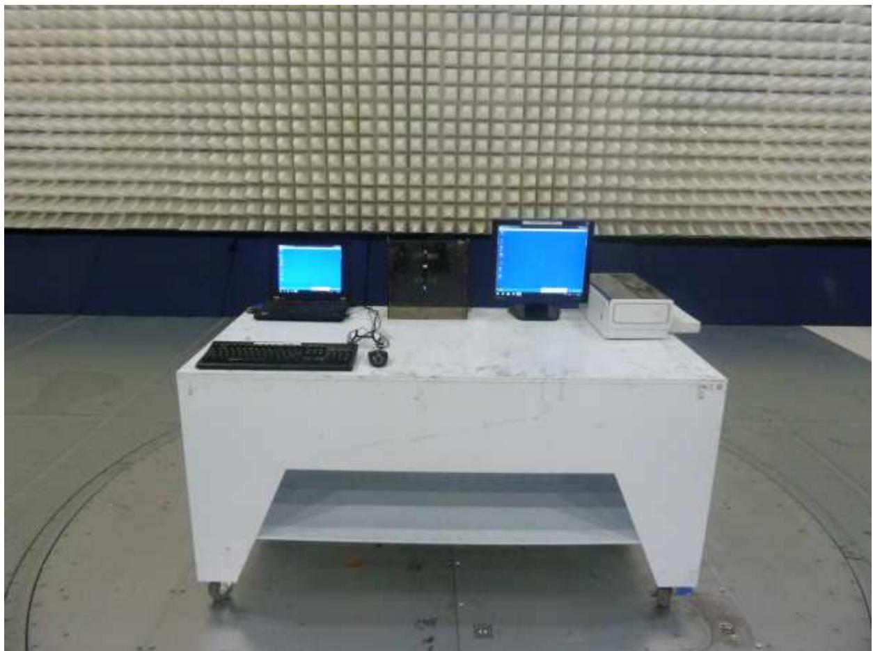
*Electromagnetic Radiated Disturbance Setup Photograph*
