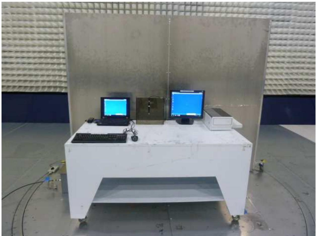
*AC Mains Line-Conducted Disturbance Setup Photograph*
