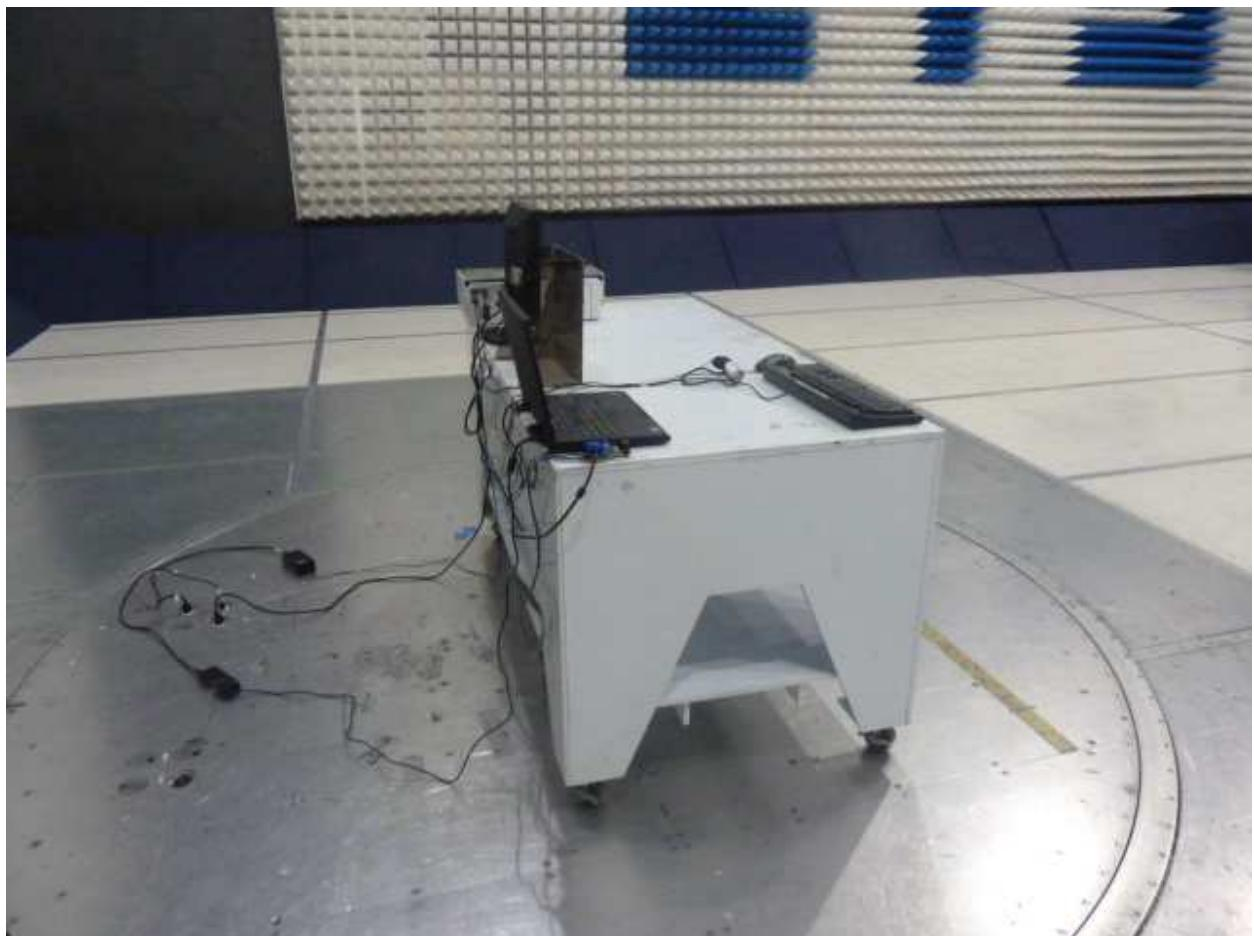
*Electromagnetic Radiated Disturbance Setup Photograph*
