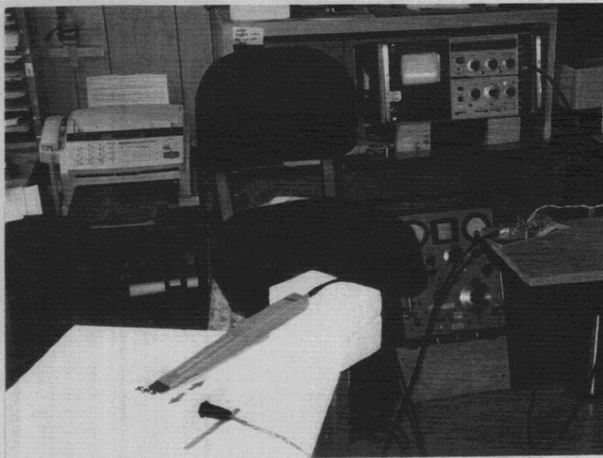
Spurious Emission Tests. 4.7 MHz to 1000 MHz. Close Field Probe
