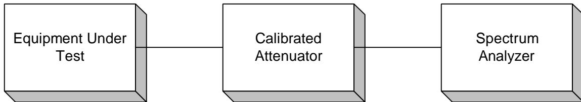
**Para. No. 2.1053 - Field Strength of Spurious Radiation**
