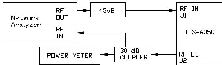
14. Turn PIN Attenuator bias voltage to maximum at FL2 of the PIN Attenuator Module. Measure the open loop gain of the booster. (Note: compensate for the 30 dB coupler). Verify that the open loop gain is within specifications. Reset PIN Attenuator voltage for 4.0V at FL2 of the module.
