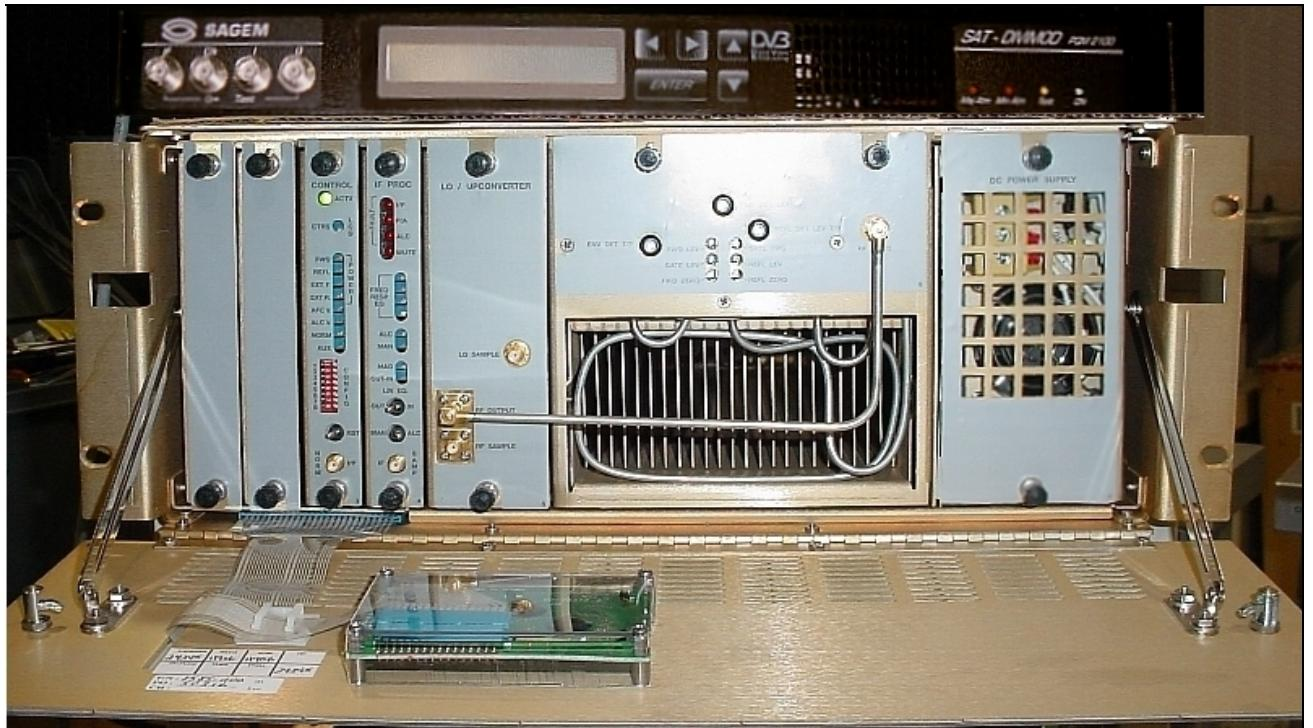
**2.3 Rear view, complete Axcera-5721 Transmitter w/Sagem QAM Modulator, Model PQM 2100**
