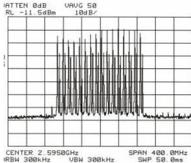
**Out-of-Band Power Plot/500 MHz Span (25.0 Watts total average):**
