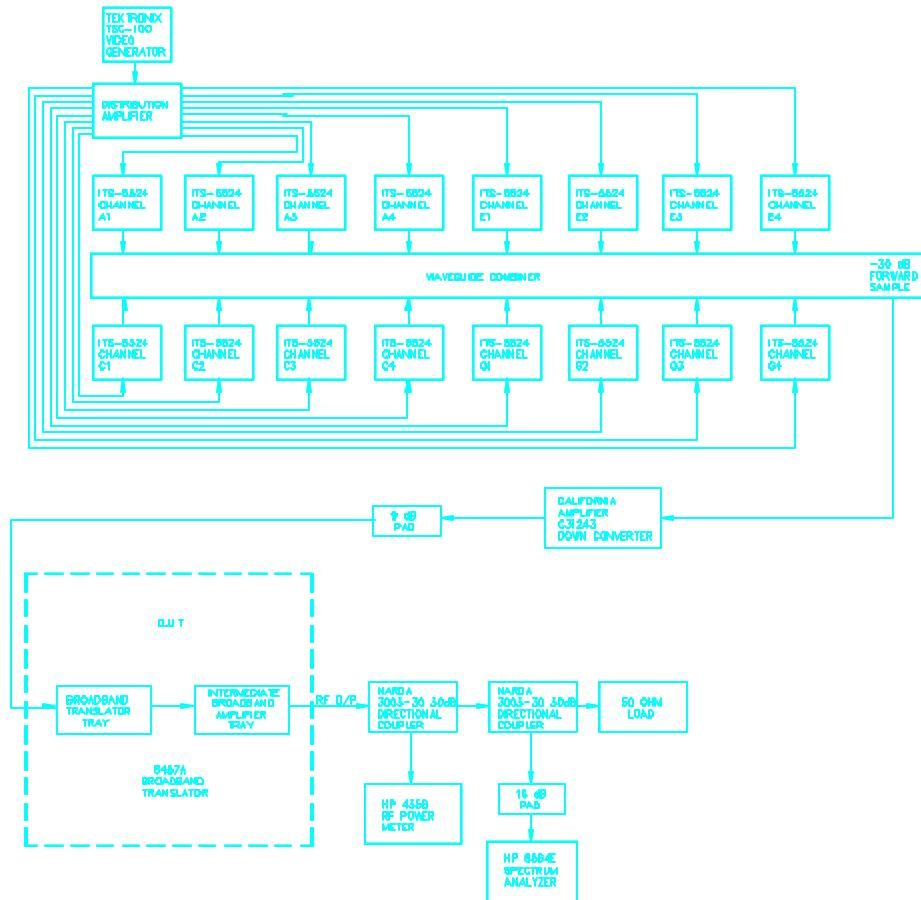
Before testing the 6457A multi-channel translator, the ITS-5724 transmitters (FCC ID# CJJ79SITS-7022) used to generate the multi-channel input signal to the translator were tested and observed to meet specifications. Then, the translator was tested and observed, as illustrated in the following sections, to reliably reproduce the transmitted signals in accordance with the rules set forth in the Rules and Regulations.
