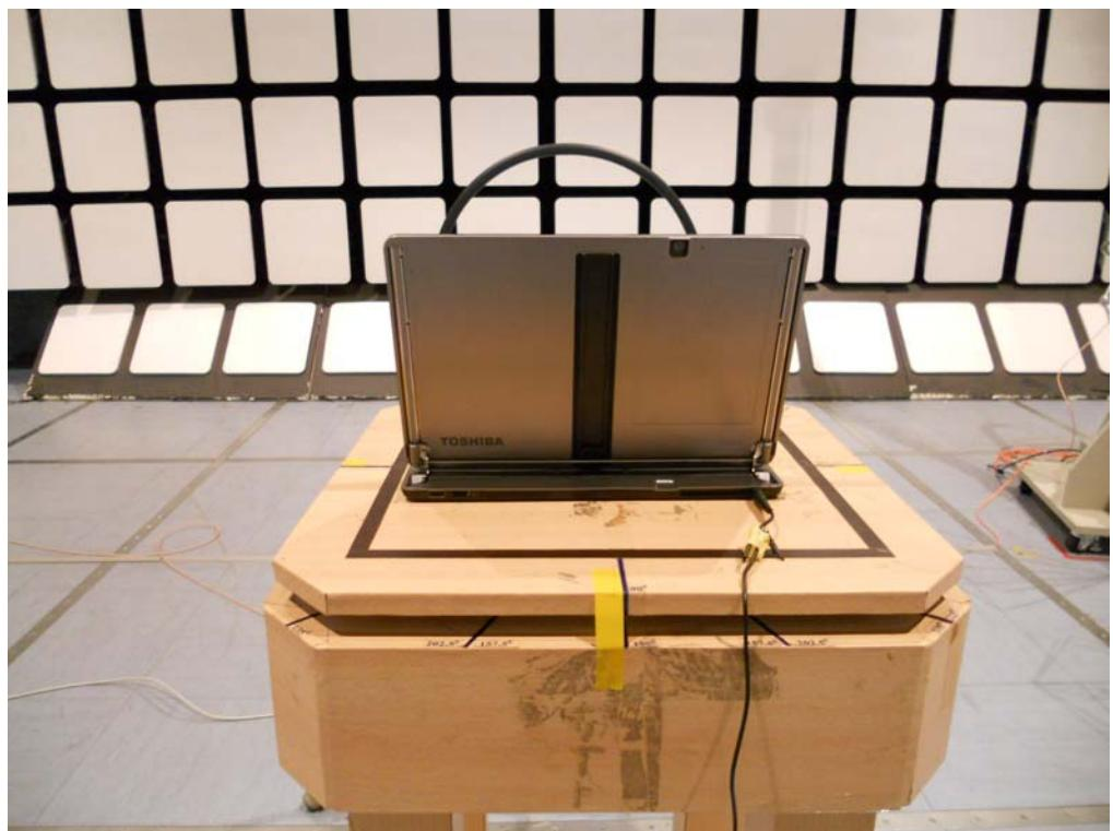
For radiated emissions 9kHz~30MHz
