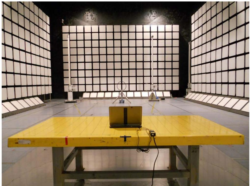
For radiated emissions 30MHz~1GHz
