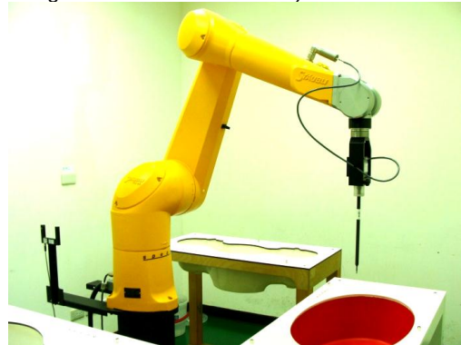
Fig 5.6 Photo of DASY5
