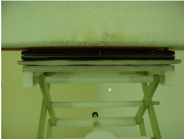
Bottom Face of Tablet with Phantom 0 cm Gap
