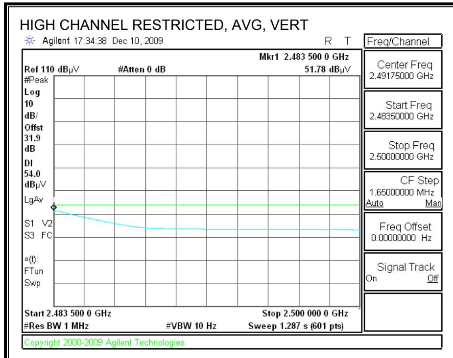
**7.2.6. 802.11n HT20 MODE IN THE 2.4 GHz BAND\_CHAIN B**
