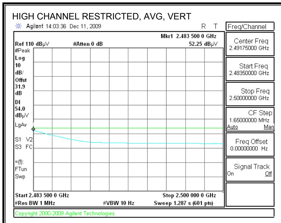
**7.2.7. 802.11n HT20 MODE IN THE 2.4 GHz BAND\_CHAIN A+B
