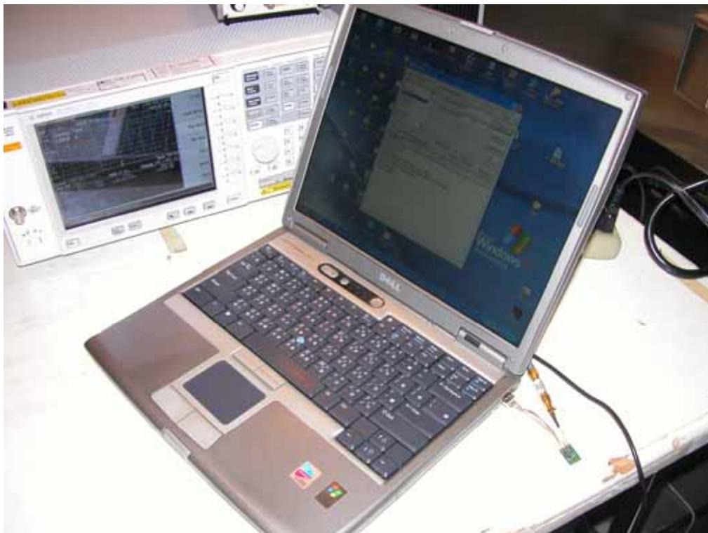
**POWERLINE CONDUCTED EMISSIONS MEASUREMENT SETUP**
