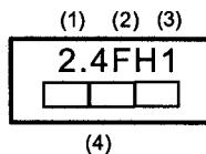
1 2.4: This equipment uses a frequency of 2.4 GHz.
